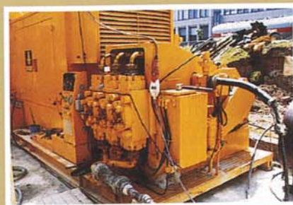
Jet Grouting Pump
